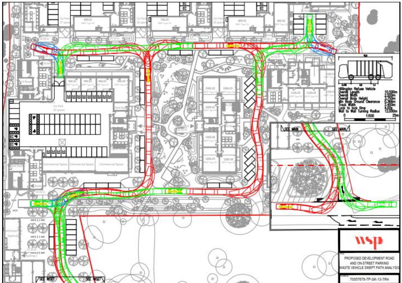
Figure 3-2: Residential waste collection with LBH refuse vehicle swept path analysis
